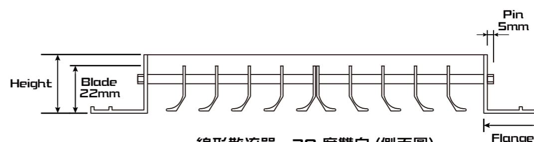
線形散流器 - 30 度雙向 (側面圖) 30 Degree Two Ways Linear Diffuser (Side View)
